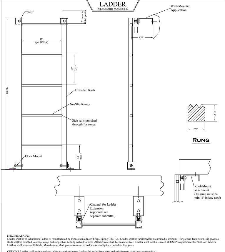
OPTIONS: Ladder shall include pull-up ladder extensions in one (both rails) to facilitate entry and exit from pit. (see separate submittal)
