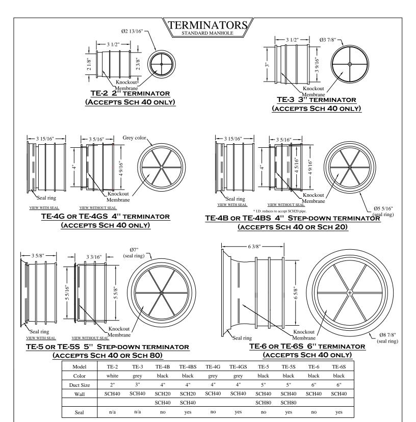
Specifications: Penetrations for cables shall be Electric/Telephone Duct Terminators as manufactured by Pennsylvania Insert Corp., Spring City, PA. Terminators shall be sized to accept 2" (3", 4", 5", 6") Sch 40 (20, 80) pipe and will provide a bonding surface for glueing cable or duct to the terminator, creating a watertight penetration. Terminators shall be manufactured from polyethylene or polyvinylcloride (PVC).
